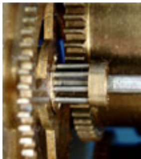
Lantern pinions are made with wires, not solid steel.
