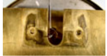
Note the straight-sided cutout with a curve at the bottom.
