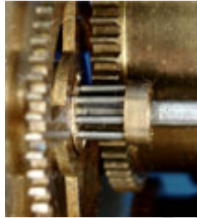
Lantern pinions are made with wires and not solid cut teeth.
