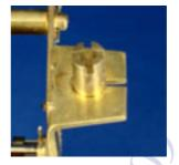
Most simple suspension supports use a pin through a hole in the support to retain the top block. This one uses a fixed top pin, which sits in a slot in the top.
