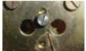
Note that the top guard screw is below the anchor pivot hole on the late model
