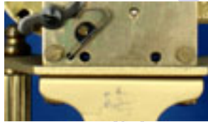
On the 8" dome model there is no gap between the platform and the movement
