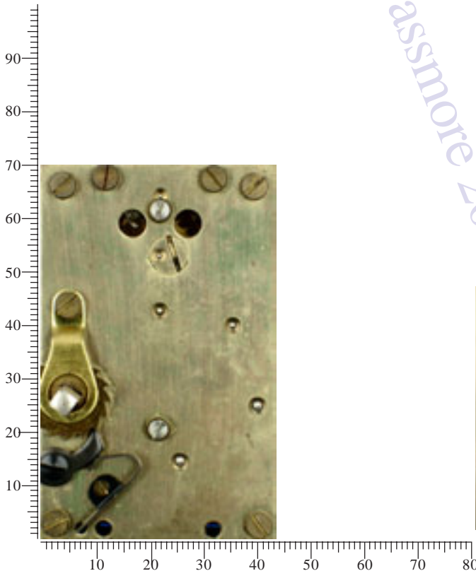
Note that the top guard screw is below the anchor pivot hole on the late model
