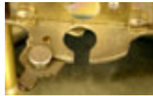
The Kundo locking device, used from this movement onwards.
