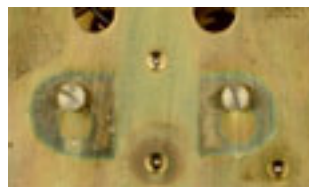
Screw holes for the earlier suspension guard.
