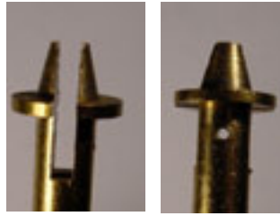
The pendulum is pinned in position with a grub screw.
