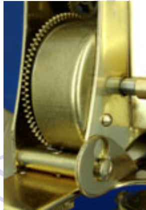
The loop end spring is inside a cover riveted to the backplate.
