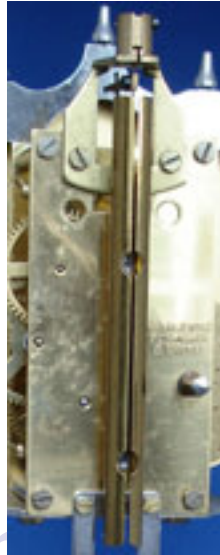
Metal guard fixed with two screws
