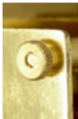
Back plate secured by serrated nuts.
